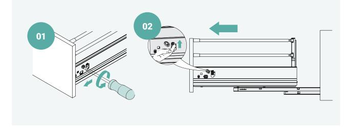
When reinstalling, push the drawer fully in to engage the soft close mechanism.
