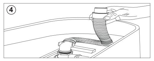
You can connect to it with a flexible drain pipe which enables you to tilt the bath up and move the bath into the required position. To avoid water retention in the trap the flexible pipe should have a continuous downward flow.
