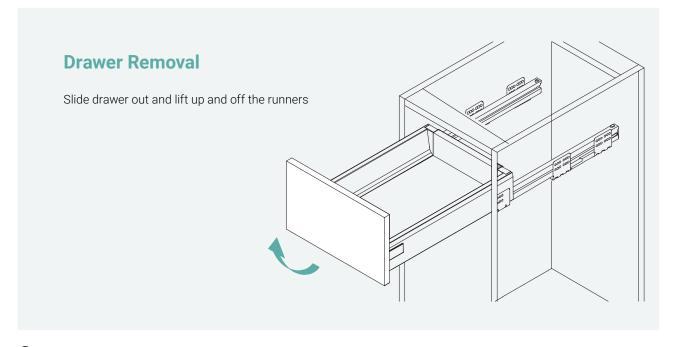
• When reinstalling, push the drawer fully in to engage the soft close mechanism.
