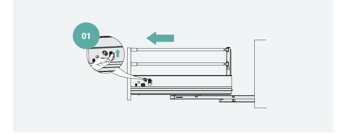
• When reinstalling, push the drawer fully in to engage the soft close mechanism.
