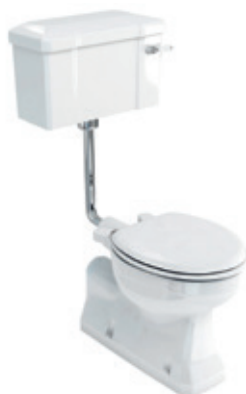
S trap LL WC with 440 lever cistern 3 star WELS rating W 450 | D 740 | H 920-1070 Pan Height 425
