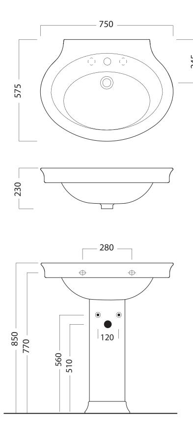
NB: Drawings indicate the technical measurements only and is not a reflection of how the unit will look.
