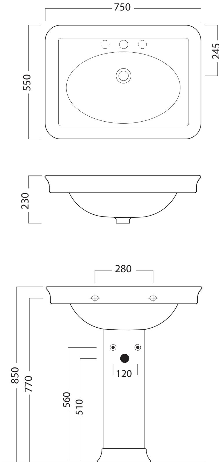
NB: Drawings indicate the technical measurements only and is not a reflection of how the unit will look.
