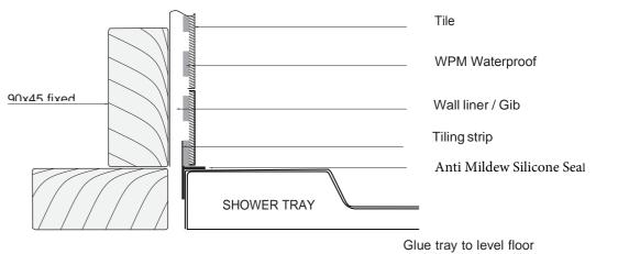
VCBC shower installation with a factory fitted upstand for an acylic liner or a tiled wall
