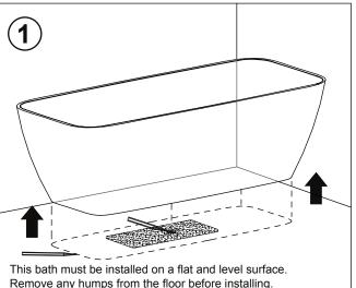
Under floor access required for plumbing of bath waste.
