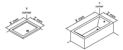
B) Cut tiling bead to required length X + Z, and make two 45° cuts at the position point Y.
