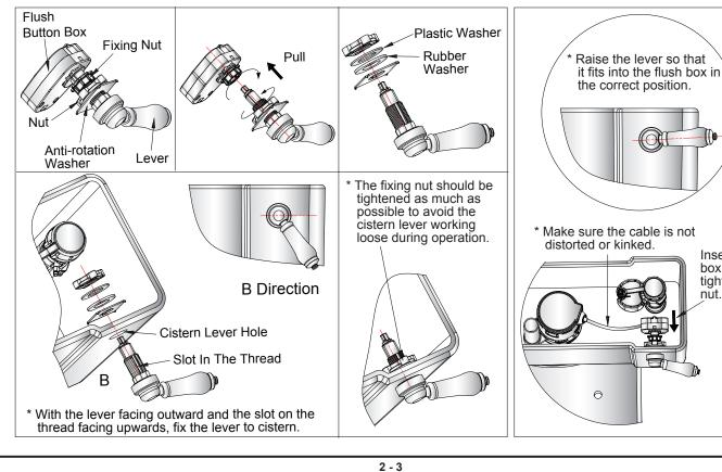
Insert the box and tighten the
