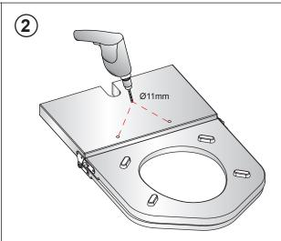
Turn the seat over, and place on a protective mat. Drill holes (recommended depth 15mm) in the marked positions using the  $\varnothing$ 11mm drill bit.
