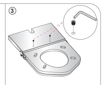
Fix the plugs supplied into the drilled holes using the allen key.
