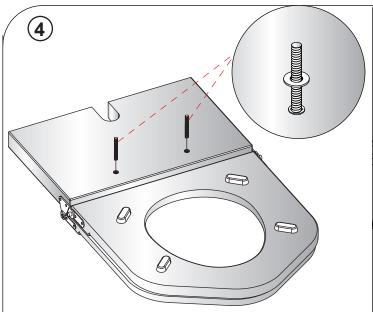
Screw the fixing bolts into the plugs, and attach on the washer.
