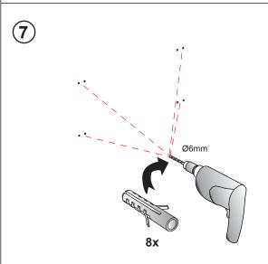
Drill holes using the Ø6mm drill bit following the marked positions, and insert the wall plugs.
