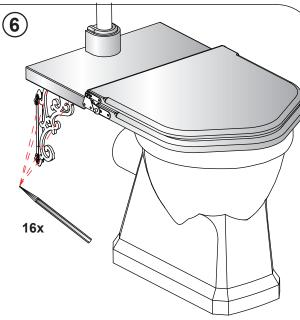
Place the ornate bracket into the fit position. Mark the fixing hole positions onto the wall and the seat by pencil.
