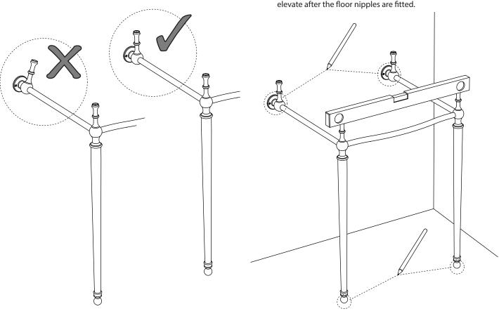
Using a  $^{1}\!/_{\!4}{''}$  drill bit drill the six holes on the marked positions. Note: In the event that the wall / floor fixings supplied being inappropriate for the wall / floor, please source alternatives.
