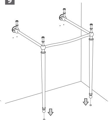
Fit the two legs over the floor nipples.
