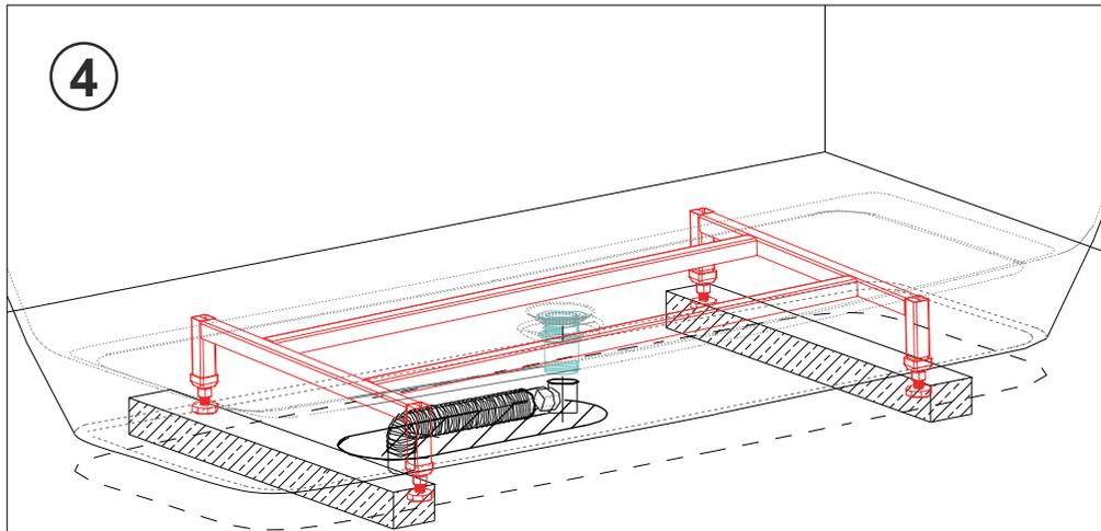
Place the bath on two wooden blocks over the waste connections. Connect the waste. Fill the bath with water and check for leaks from the waste before removing the blocks.
