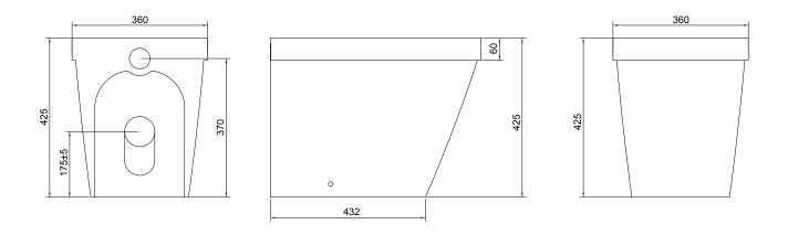
NB: 140 - 160mm S Pan. Adjustment with STC Convertor (not supplied)
