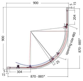
\*(15mm adjustment for easy fitting per panel)
