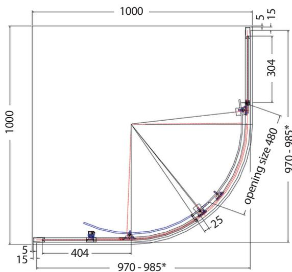
\*(15mm adjustment for easy fitting per panel)
