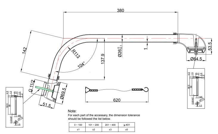
For the finished assembly, the dimension tolerance should be followed the list below.
