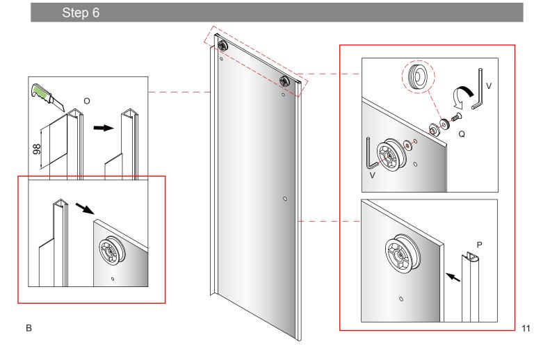
Hang the glass onto the top track. At the bottom, insert the door glass into the slot of the glass clamp (LM). Slide roller 2 to align with the fixing hole in the door glass. Use the Allen keys (U, V) to fix the roller 2 connector to the door glass.
