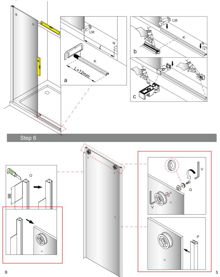
Hang the glass onto the top track. At the bottom, insert the door glass into the slot of the glass clamp (LM). Slide roller 2 to align with the fixing hole in the door glass. Use the Allen keys (U, V) to fix the roller 2 connector to the door glass.
