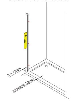
Remove wall channel from the glass panel frame. Place wall channel in position on the tray (8 - 12mm in from the outer edge of the tray), use a spirit level to ensure that they are vertical and mark all 3 fixing holes onto the wall. Make sure the lip of the tray is 70mm minimum.
