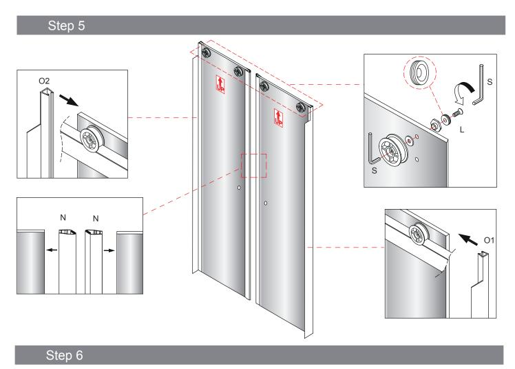
Hang the glass onto the top track. At the bottom, insert the door glass into the slot of the glass clamps (GI, HJ). Slide roller 2 to align with the fixing hole in the door glass. Use the Allen key (T, S) to fix the roller 2 connector to the door glass.
