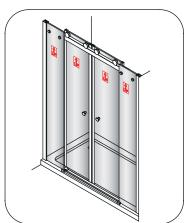
• The "up" arrow on the sliding door should be above, and be on the outside of the enclosure.
