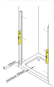
Remove both wall channels from the glass panel frames.
