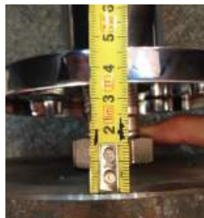
Note: Under some pressure the sticking out length can be reduced to 35mm.
