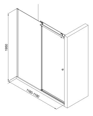
\*30mm adjustment for easy fitting per panel
