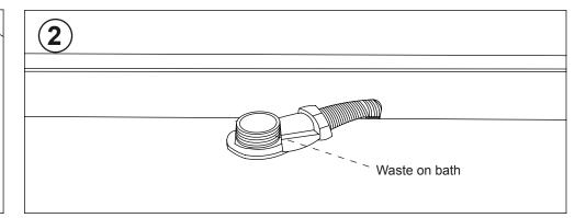
The baths have no panel to remove for access to the waste.
