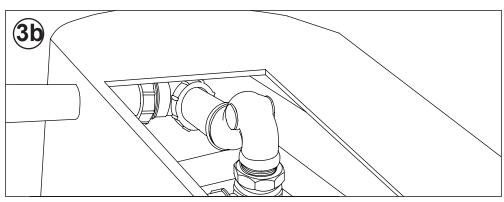
Method 2) If under-floor access is impossible, an additional hole of approx 45mm diameter can be drilled through the outer skin of the bath to allow the trap to be connected to a rigid pipe.
