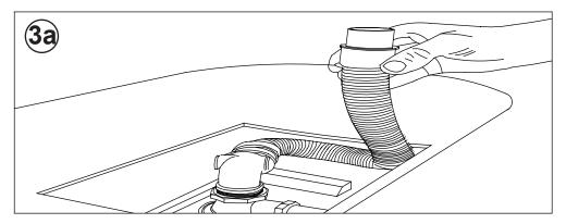
Method 1) If you have a waste that comes up through the floor, you can connect to it with a flexible drain pipe which enables you to tilt the bath up and move the bath into the required position. To avoid water retention in the trap the flexible pipe should have a continuous downward flow
