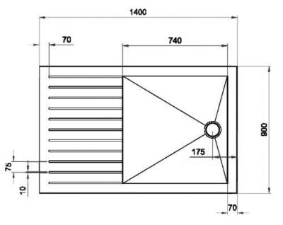
NB: Drawings indicate the technical measurements only and is not a reflection of how the unit will look.
