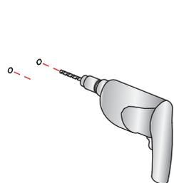
Using a 6mm drill bit, drill holes on the marked positions.
