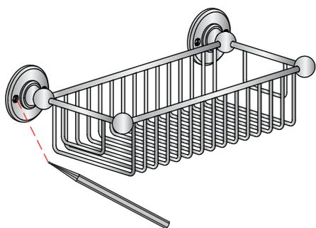
Determine the final installation position, mark the fixing hole positions in pencil.
