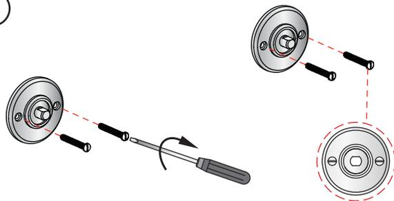
Screw in the stainless steel screws to secure the base to the wall. Please ensure that the screw heads are parallel to the floor.
