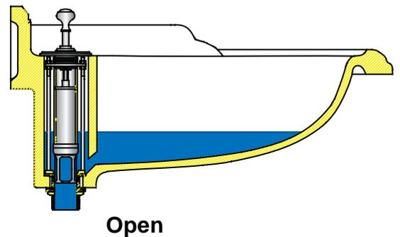
To operate the waste lift and turn to open , lift and turn to close.
