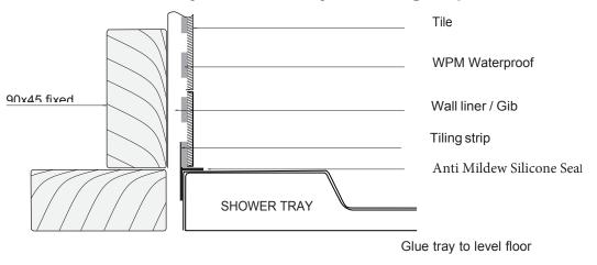
VCBC shower installation with a factory fitted upstand for an acylic liner or a tiled wall
