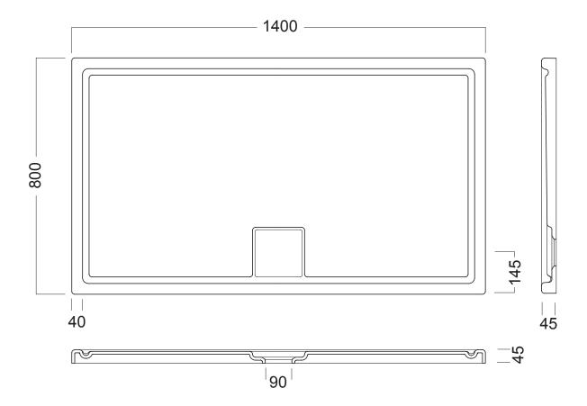
NB: Drawings indicate the technical measurements only and is not a reflection of how the unit will look.
