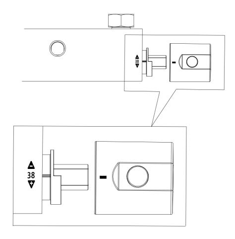
Step 3:. Put the valve covers and handles back on and ensure the etching on the valve cove aligns with the mark on the cartride and etching on the handle.
