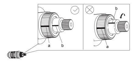
Step 1: Align the black marks on part a and b.
