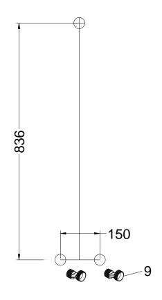
② Insert the plugs (3) into the wall, fix the wall bracket (4) with the screw (5) on the wall and mount the mixer(12).
