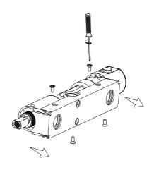
Step6: Remove the grub screw and take out the cartridge.
