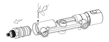
Step 7: Put the new cartridge into the valve body, and put the covers, stop limit and handles back in sequence. Set the temperature (refer to section "Temperature Setting).
