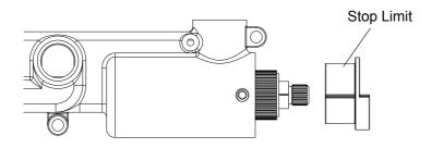
Step 2: Put the stop limit back onto the cartridge. Ensure that the black mark on the stop limit aligns with the mark on the cartridge.
