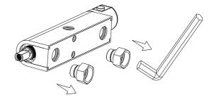
Step 4: Separate the valve cover from the valve body.
