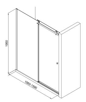
30mm adjustment for easy fitting per panel
