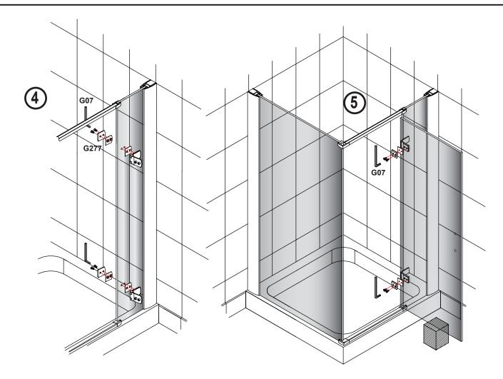
Make sure the hinges have been tightened securely during installation.
