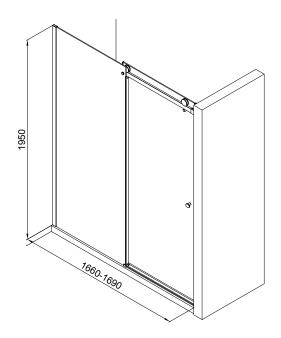
30mm adjustment for easy fitting per panel
